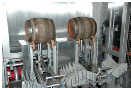
Pic. 4: Once a barrel is on the grippers, the cleaning process runs fully automatic at the push of a button.
