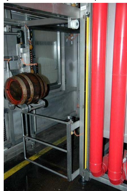
Pic. 6: Guarding with SOLID-4E Safety Light Curtains allows the barrel to be safely removed at the system exit after cleaning.
