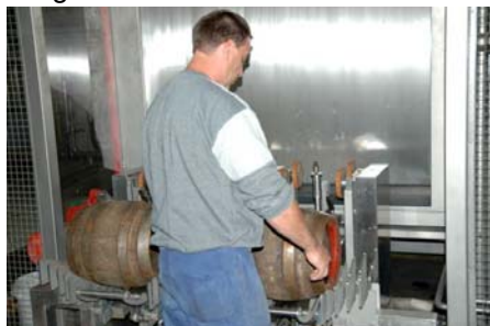
Pic. 3: Guarding with integrated SOLID-E Safety Light Curtains means the operator is no danger when feeding the wooden barrels.
